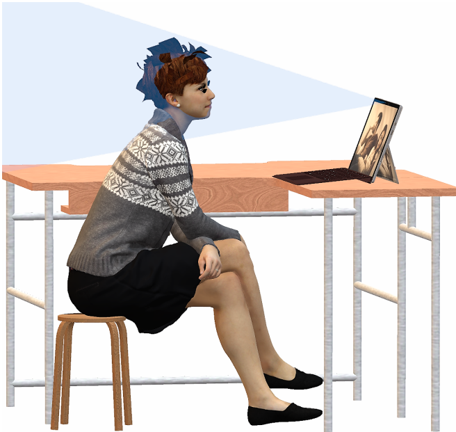
Figure 2. Taking the BAT v2 test on a Microsoft Surface Pro 4 tablet. Using only the integrated webcam and microphone, BAT v2 is capable of extracting reliable HRV features, facial expressions, linguistic and paralinguistic features of speech, gaze, and head movements.
